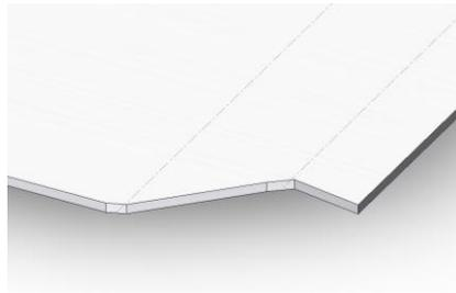
The ending of the flange and the bend zone can be seen as single plane faces.
