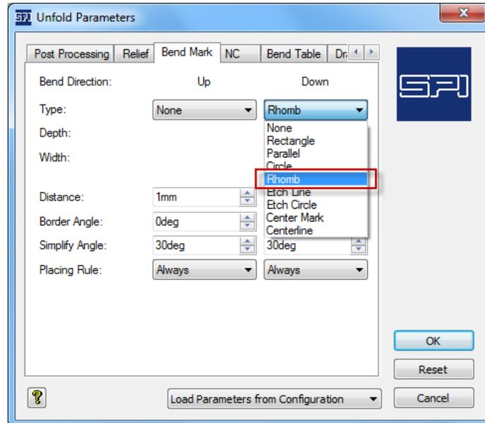
When selecting *Etch Line* or *Etch Circle* as bend mark type, the bend marks will only be created as small sketch elements. *Rhomb* will put small notches into the contour at the end of the bend lines:
