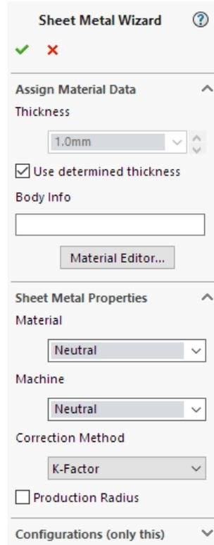
The thickness is obtained from the geometry automatically. If this thickness is not the correct one you may enter the correct thickness or determine it by selecting a face. For this uncheck the option *Use determined thickness*.
