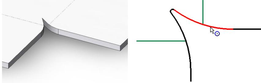
The corner is composed of two splines that meet in one point.
