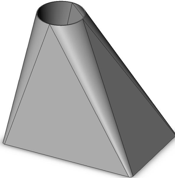
In some cases it is necessary to increase the values for the precision on the tab **Freeform Surface** within the **Unfold Parameters**.
