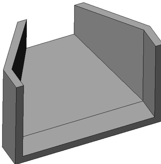
**2<sup>nd</sup> Shelling with desired thickness**
