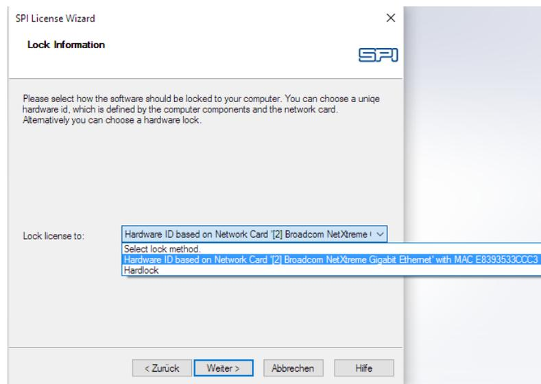
Besides attaching the license to the unique *Hardware ID* of the computer it is also possible to use a *Hardlock*, also known as a dongle. An USB dongle can be ordered with costs at SPI. This will allow using one license on more than one computer, for example in the office and at home.
