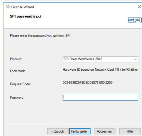
When you receive the unlimited password, you can launch the SPI License Wizard at any time within the **About SPI SheetMetalWorks** dialog and enter the password.
