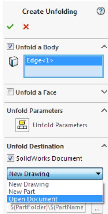
Since the part has been unfolded before, the **Unfold Destination** is preset to *Update*. Toggle the **Unfold Destination** to *Open Document* and choose the drawing file.
